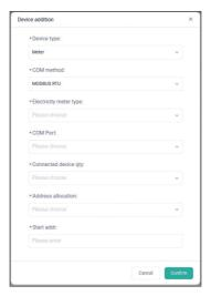
Figure 6-12 Adding meter through Modbus RTU
