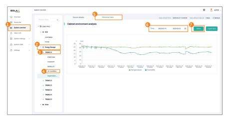
Figure 6-69 Checking the cabinet environment analysis
