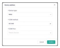
Figure 6-13 Adding meter through DLT/645
